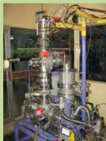
Fig. 3. The self-developed vertical compact ion implanter. Its total length, from ion source to target chamber, is only 1.36 meters.
