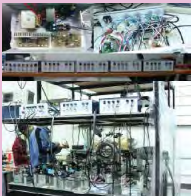
Prototype diode laser systems for atomic physics, (top) driver and servo-lock, (middle) five control systems and (bottom) all lasers at different frequencies in operation.
