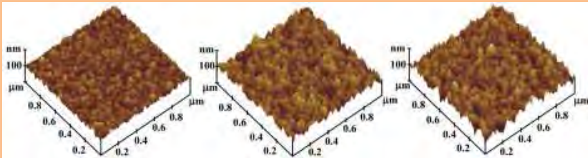
AFM of TiVN films deposited at different sputtering currents.
