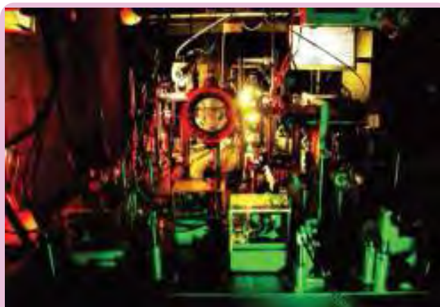
Thailand cold atom facility. The system is capable of producing 10^9 rubidium atoms at temperature \sim 145 \mu\text{K} in less than 2 s. Cold gas is a starting material in various experiments.
