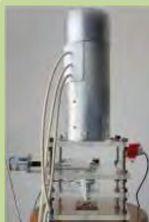
Fig.1. The home-made ion beam deceleration lens. The lens of only 22 cm long is capable of reducing ion energy from 30 keV down to 20 eV with a beam current up to \mu\text{A} .
