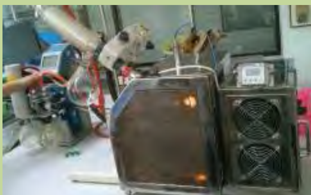
Low pressure microwave evaporator.
