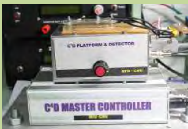
Fig.7. The self-developed MCE-C 4 D system with plug-in MCE device at the top.
