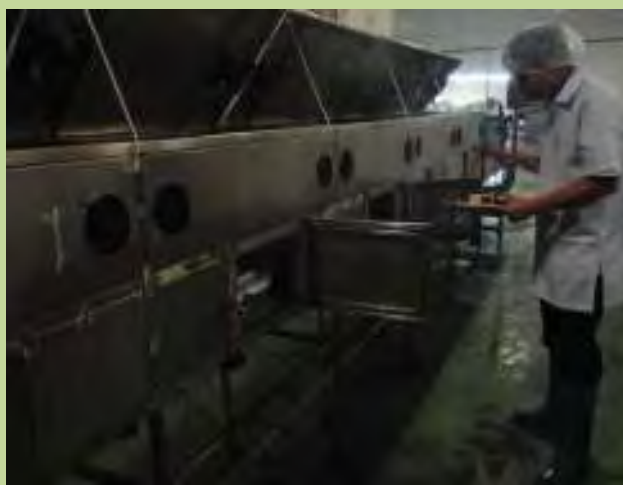
Conveyor microwave heating system for food industry.
