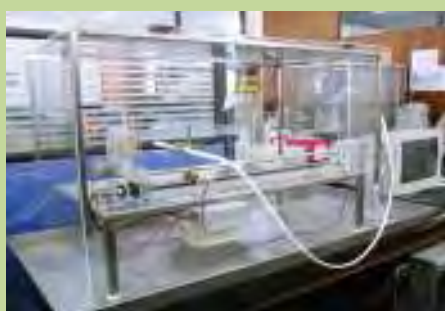
A picture of polymer spray-coating system for tubular ceramic membranes.
