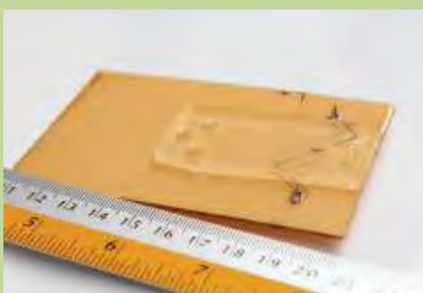
Fig.6. Low cost single use PDMS based MCE device designed and fabricated by our group.
