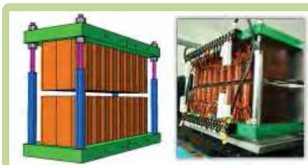
Prototype of a undulator electromagnet with \lambda_p = 55 mm.
