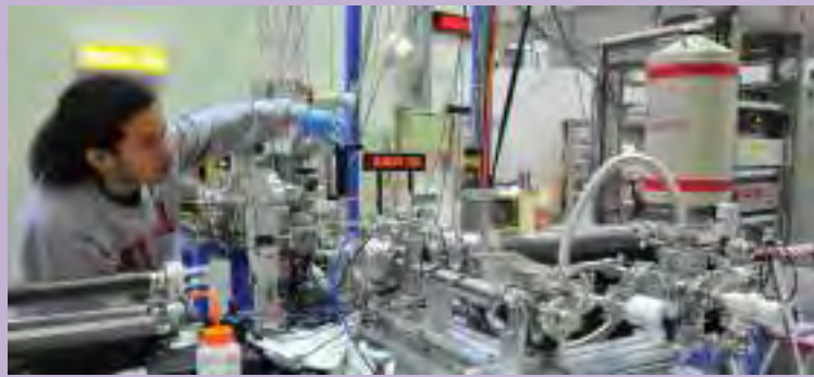
X-ray absorption spectroscopy experimental station at the Synchrotron Light Research Institute. The experimental station was employed for XANES measurement for determination of the local structure of matters.
