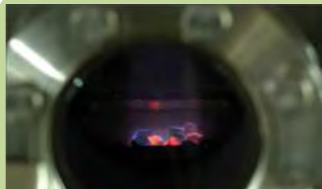
Fig. 4. Luminescence of gemstones while being irradiated with nitrogen ion beam generated from the implanter shown in Fig. 3.
