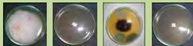
Fungal tolerant tests on cellulose membranes, before and after electron beam irradiation.
