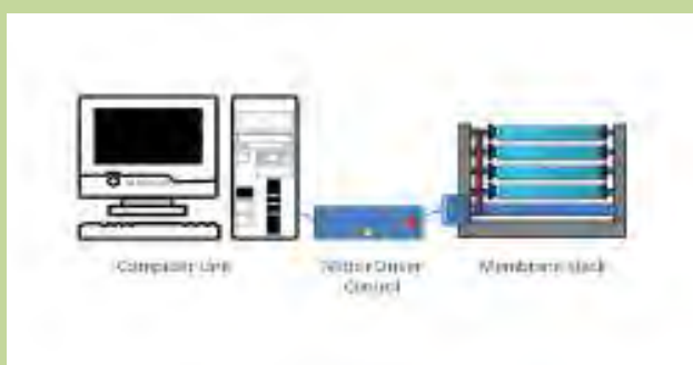
Diagram showing a control system for polymer spray-coating on ceramic membranes. (a) Electronic control system (b) Ceramic membrane holders attached with a rotation control system using a step motor.
